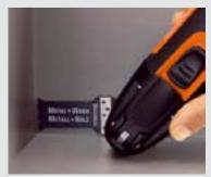
Make cut-outs for cable inlets, sockets and plumbing connections using the E-CUT saw blades – without time-consuming dismantling.
