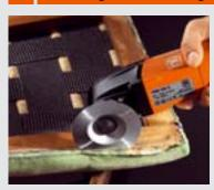
The flush cut HSS saw bladesaves you effort and the upholstery, as staples can be easily removed and do not have to be pulled out with pliers.
