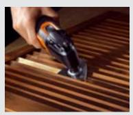
The flat sanding pad also gives access to tight spaces, e.g. the slats of shutters.
