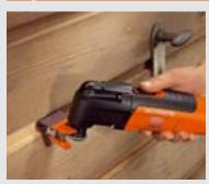
The FEIN MULTIMASTER with the profile sanding set is ideal for sanding garage doors, tongue and groove boards and other concave and convex profiles.
