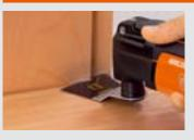
The FEIN MULTIMASTER requires very little strength to operate, removing old floor coverings and cutting parquet or laminated flooring, undercutting boards and door frames easily.
