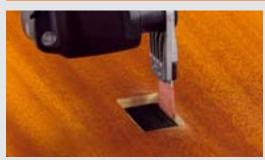
With the new carbide file insert for the MINICUT and file set, grooves can be filed out cleanly, and wood and plastic completely deburred.
