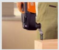
Saw into wood 2 3%" deep with the new universal E-CUT saw blades.
