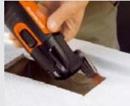
Recesses can be filed precisely to shape with the MINICUT and File Set.
