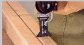
The tried and tested universal E-CUT saw blade is now available in the wider 1 3/4" design. The saw blade can be used with or without depth stop.
