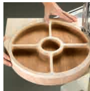
Bandsaw the exterior to final shape.
