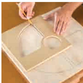
Trace the templates onto the bowl blank.
