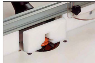
Zero Clearance Inserts for safer, more accurate routing.
